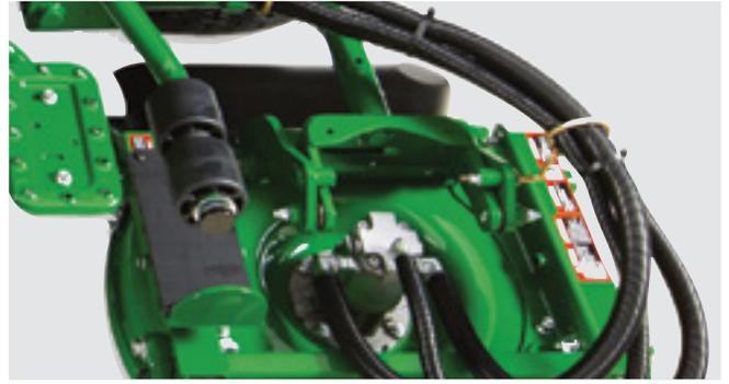
The double yoke on the 9009A means the rotary decks follow the contours in the most undulating terrain for an exceptional quality and consistency of cut.
