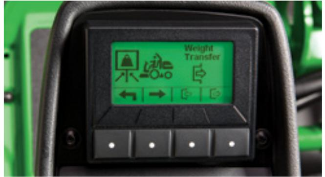
Passcode-protected TechControl display lets you precisely set mowing speed, turning speed, or transport speed for consistent performance.
