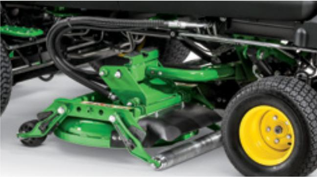
Our unique rear deck design allows for greater clippings dispersion and the deeper shell stands grass up for an even cut.
